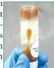
encouraged by the initial laboratory test, commissioned a comparative bench-scale test using a client's soil sample that contained concentrations of VOC's, lindane and 1,4-dioxane (see table 2). The results of this laboratory test confirmed the previous test results and concluded that the ISOTEC MFR process is successful in treating 1,4-dioxane to levels below regulatory MCL's.
